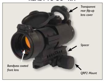
Flip covers are induded to further protect the lenses, and a transparent rear lens cover is utilized allowing the user to engage a target with the lens covers dosed in an emergency situation. Both the front and rear lenses are recessed within the sight body to provide protection against impact damage, scratches, and fingerprints.
